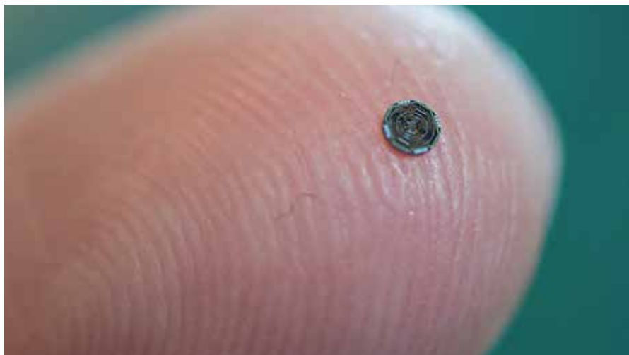
The George W Woodruff School of Mechanical Engineering is developing minute systems that can be mounted on a catheter used to find blockages in arteries (Photo: Georgia Tech)
