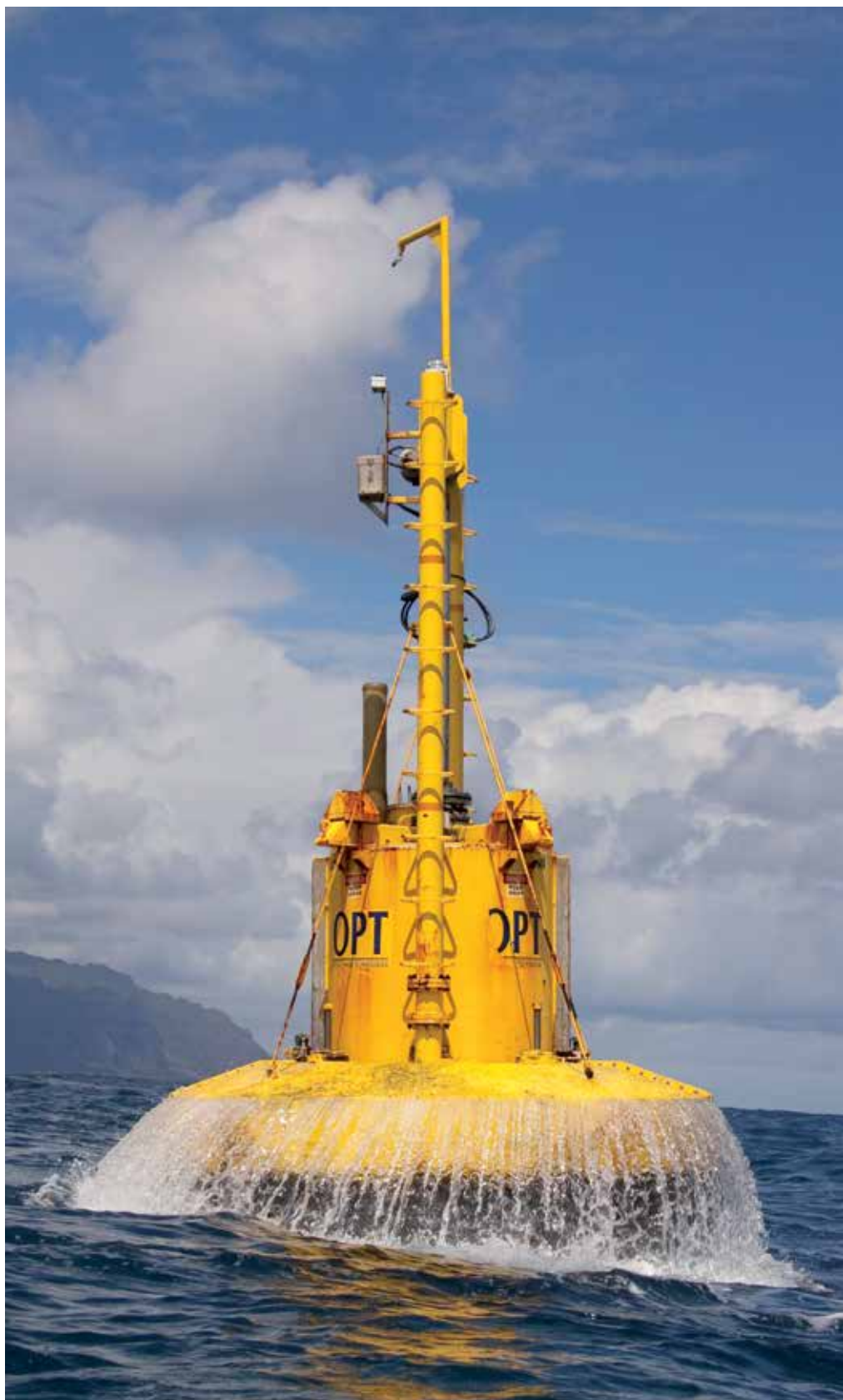
This powerbuoy draws electrical energy from the ocean's waves (Photo: Lance Cpl. Vanessa M American M)
