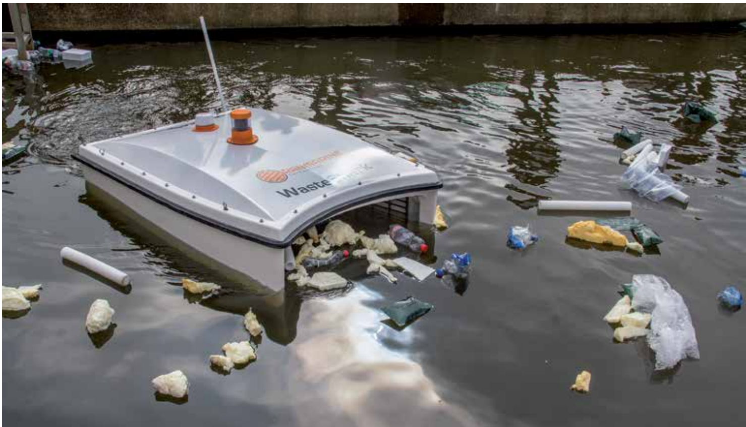
WasteShark autonomous waste collection drone designed to tackle the problem of marine litter (Photo: RanMarine Technology)
