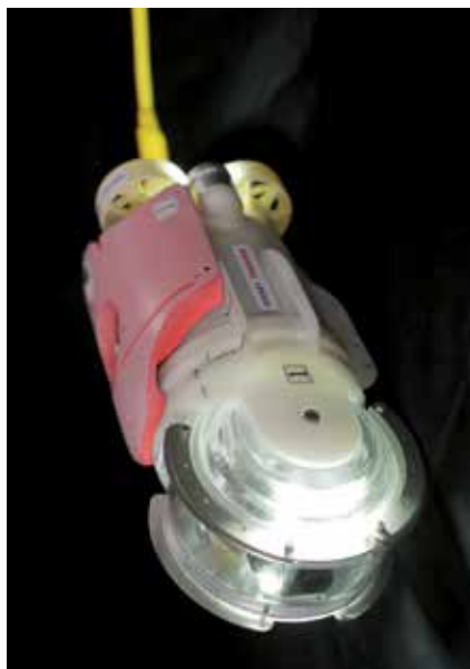
Small, radiation-hardened screw-driven submersible robot developed by Toshiba and the International Research Institute for Nuclear Decommissioning to inspect the interior of the primary containment vessel at Fukushima Daiichi 3 (Photo: Toshiba)
