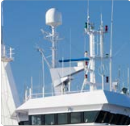
Radio and satellite communication aerials on a ship
