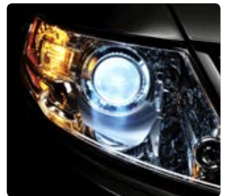
Xenon has a higher lighting capacity than traditional halogen lighting [source: Lincoln MKS]
